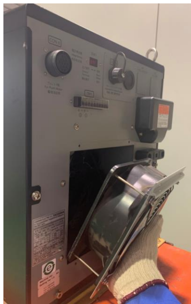
Fig. 4-2: Preparation for Pulling out the Fan Cable
