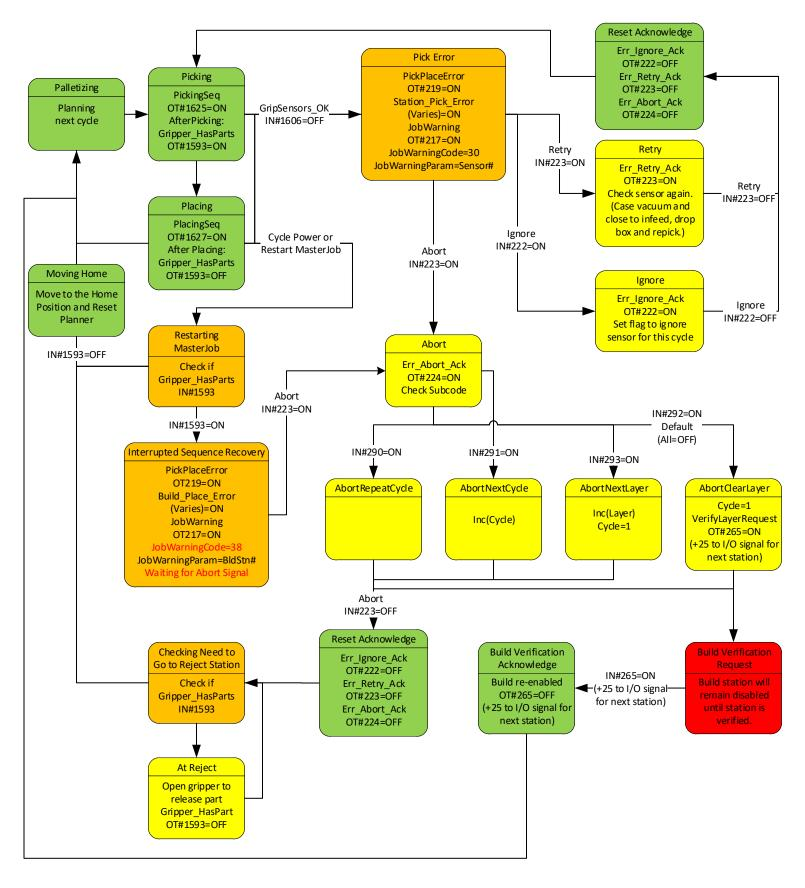
NOTE: Essentially the same diagram applies also to pallet and slipsheet pick/place sequence except for the Signal GripSensor\_OK IN#1606 is replaced by IN#1597 to 1600 depending on the selected dispenser.
